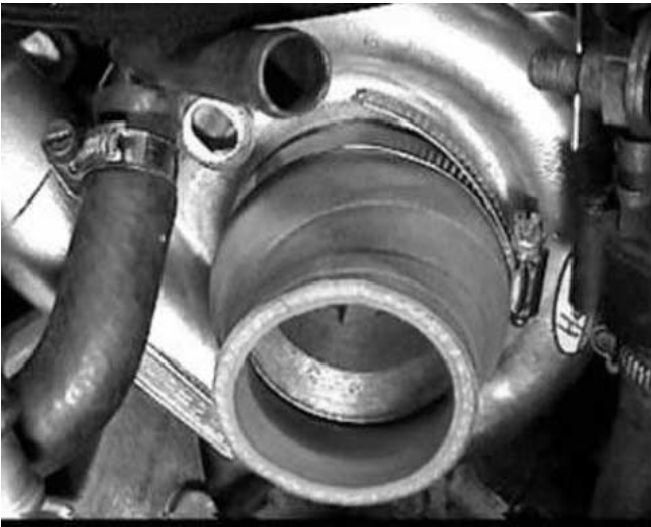
• Above - New Turbocharger in place
